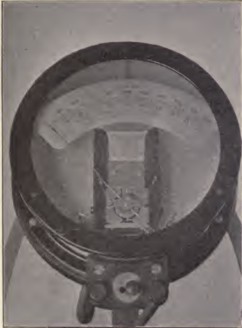
FIG. 10.—Massey Type Weston Milliampere Meter. The divisions of the scale may be seen some yards from instrument, and extend, on the two scales, from 0 to 100 and 0 to 2000 milliamperes, being capable of being read to 1-2 milliampere. To select scale place plug in appropriate socket shown in lower portion of cut.
